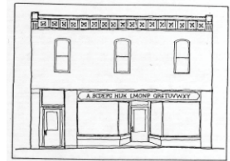
PLACEMENT OF SIGNAGE ON FASCIA
