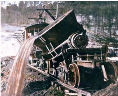
25 ton cast-iron pot dumping molten slag. Slag is the waste product of the copper smelting process. Photo: Greenwood Museum P366
