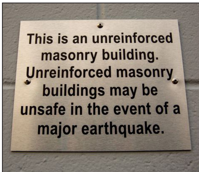
Fig. 5.7: Example of a seismic hazard sign installed on URM buildings in California. (Source: Courtney Sherwood)
